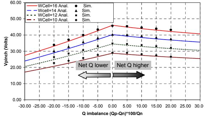
Figure 5. Comparison of Analytical & Simulated  $V_{Pinch}$  as a function of % column charge imbalance for  $Q_N = 1.5e12 \text{ cm}^{-2}$
