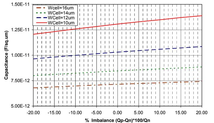
Figure 6. Simulated Zero Bias Junction Capacitance  $C_{J0}$  as a function of % column charge imbalance for  $Q_N = 1.5e12 \text{ cm}^{-2}$
