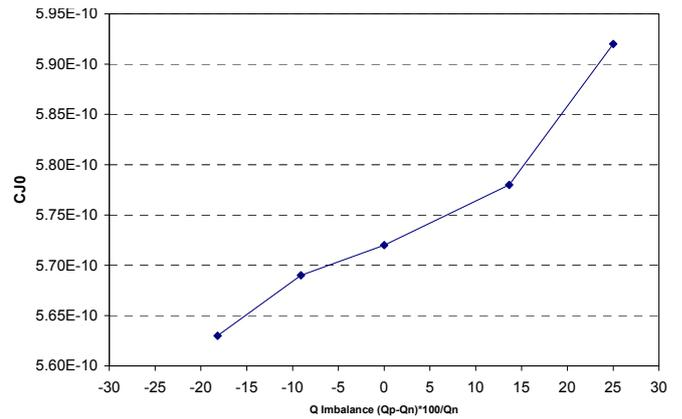
Figure 9. Measured  $C_{J0}$  vs P Column Dose on Fabricated 600V Super Junction MOSFETs
